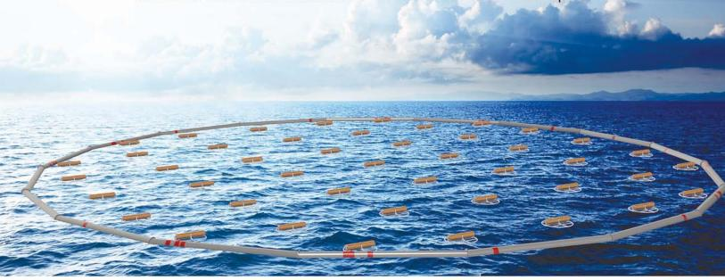
Means: The deployment of 70 m diameter large ring containing 3000 high-precision temperature sensors distributed over 45 vertical lines 125 m high and 9.5 m apart. The sensors measure water temperature with a precision better than  $0.0005^{\circ}$ C, every 2 s synchronous to within  $\pm 0.01$  s. The whole fills a half cubic hectometer seawater volume. The unique mooring is expected to remain underwater for 3 years.
